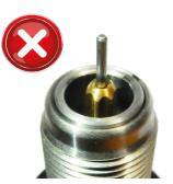
Spindle set incorrectly – The knurled sleeve extends beyond the die.
