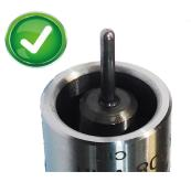
Spindle set correctly – The interior sizer does not extend beyond the die.
