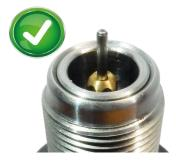
Spindle set correctly – The knurled sleeve does not extend beyond the die.
