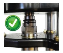
Die set correctly – The case holder does not contact the die.
